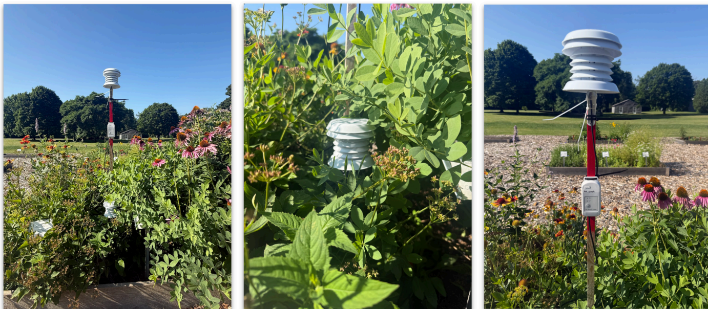
A HOBO RX 2302 bluetooth logger capturing sub hourly microclimate data in a raised garden bed. Images by Markana Cruz 2026.
